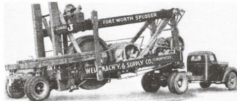
Figure 13.63 (right). Fort Worth spudder Model Super-J, 1935.
